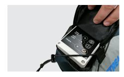
**ii.** Insert the battery charging plug unto the socket on the pump enclosure.
