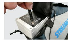
iii. Plug the charger into a 230v mains power supply and switch it on. The blue charging light on the pump enclosure will illuminate.
